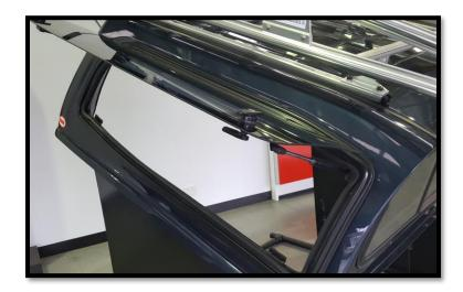
2. From the gas strut holder remove the clip using flat screw driver. Repeat on both gas struts.
