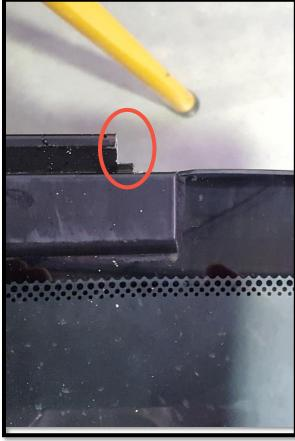
6. Replace the locks if necessary to have the same key for all of locks in the canopy. Remove the allen head screws and a nut. Replace the lock. Repeat in the reverse order for both locks.
