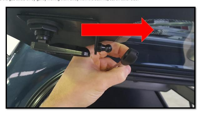
4. Lift the glass up to detach the hinge from the frame, take the glass off.
